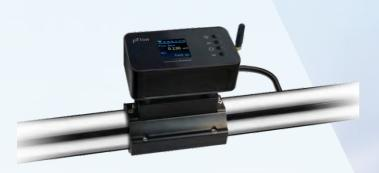
F3R adopts the principle of ultrasonic transit time measurement, combined with the patented flow algorithm technology, to make accurate measurement of fluid flow in the pipeline. The product is of all-in-one compact structure design, which makes the installation simple and convenient, only 4 steps are required. It does not contact with the fluid during installation, and the flow does not have to be shut off.
